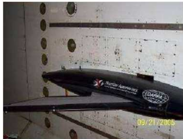
Figure 24 – NextGen model mounted in TDT
